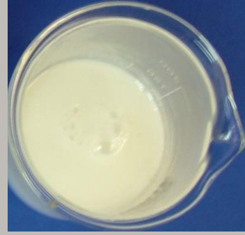
5% Dilution of Antifoam made with static mixer
