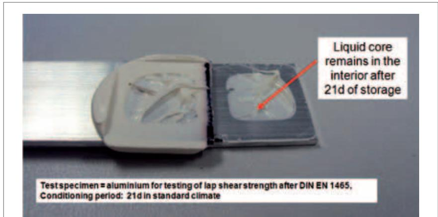
Figure 4: Example of a SPUR/SPE-based formulation for flexible bonding with incomplete cure.
