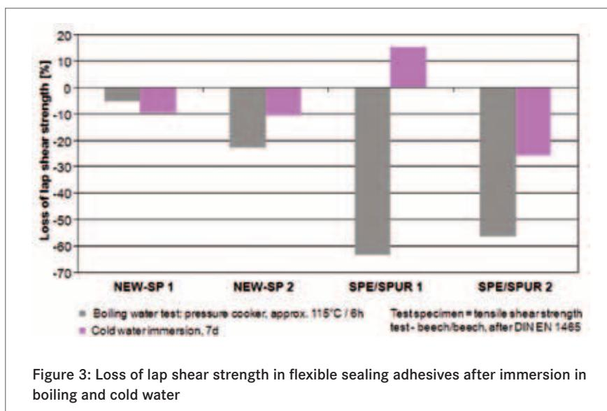
significantly lower in NEW-SP polymers than in commercially available SPUR/SPE formulations (Figure 3).
