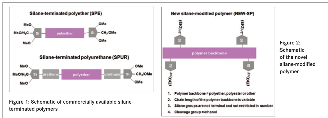
Figure 2: Schematic of the novel silane-modified polymer
