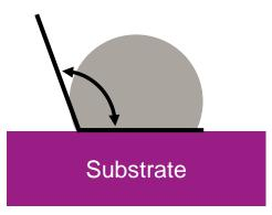
poor surface wettability surface tension (droplet) > surface energy (substrate) contact angle >90°
