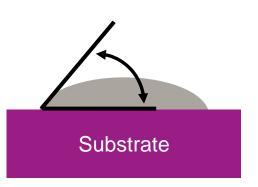
good surface wettability surface tension (droplet) < surface energy (substrate) contact angle < 90°
